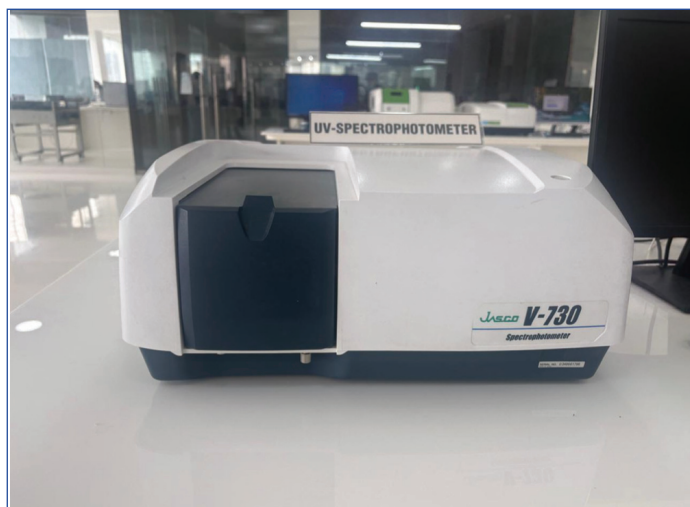
[Table/Fig-2]: UV spectrophotometer used to assess the absorbance of samples for the anti-inflammatory activity.
