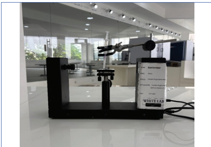
[Table/Fig-9]: Ossila goniometer for measuring the contact angle.
